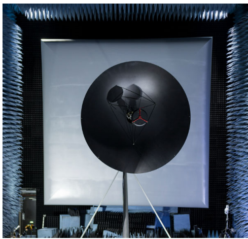
Figure 3. Flight HGA in NASA LaRC ETR
