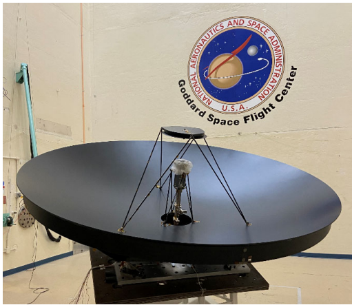
Figure 2. Flight HGA in Acoustics at NASA GSFC
